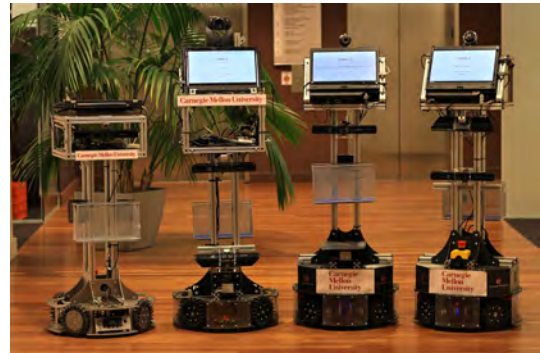
Figure 1: CoBots with omnidirectional motion, onboard computation, interaction interfaces, carrying baskets, and different combinations of depth sensing (cameras and LIDAR).
