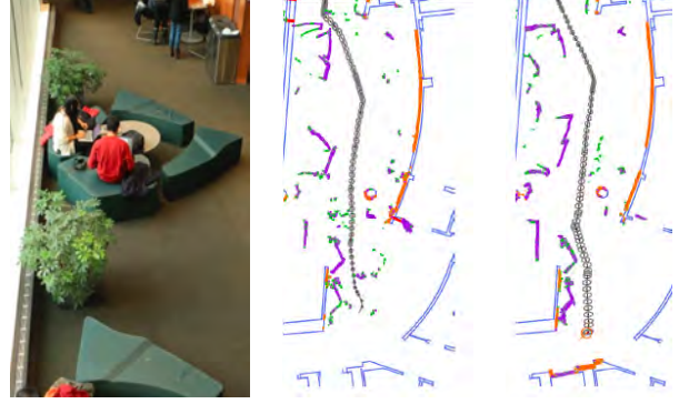
Figure 3: View of the challenging varying space in GHC4 atrium and snapshots of enML at two different times. The trajectory of the robot over the episode is shown in grey, along with the covariance ellipses. LTF observations are shown as orange points, STF observations as purple points, and DF observations as green points. The long-term static map is shown as blue lines.
